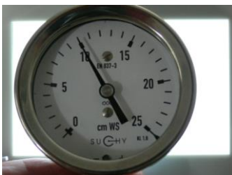
Figure 11: Manometer for pressure calibration
