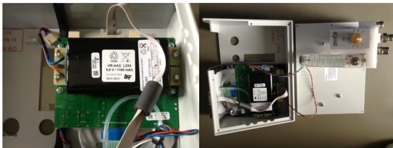
Figure 15: medinSINDI ® CPU and open housing with mixer and CPU
