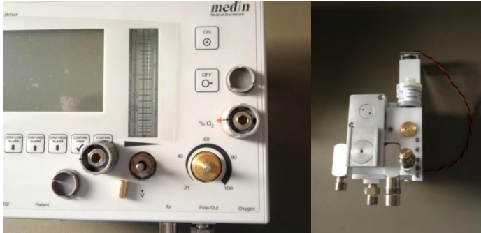
Figure 16: Disassembly of the knobs on the front panel and mixer with oxygen cell
